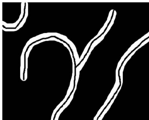
Figure 5. Artificial example to illustrate thinning where thick lines are condensed into thin “skeleton-like” lines.
